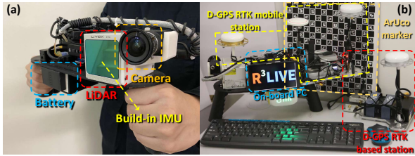
Fig. 5: Our handheld device for data collection. (a) shows our minimum system. (b) shows an additional D-GPS RTK system and an ArUco marker board used to evaluate the system accuracy.
