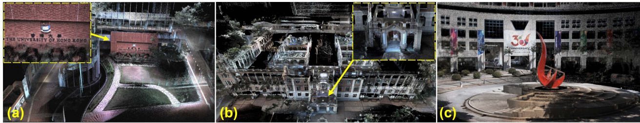
Fig. 1 – The radiance map of HKU (a and b) and HKUST campuses (c) reconstructed by R 3 LIVE++ in real-time (see our accompanying video on YouTube: youtu.be/qXrnIfn-7yA ).
